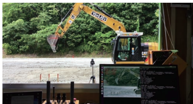
▲ Automation of excavator using deep reinforcement learning
