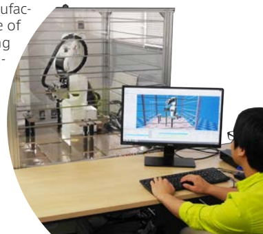
Prototype system of digital triplet for an assembly process ▲
